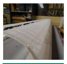
An Air Foil scale designed from architectural drawing files and manufactured for the Boundary Layered Wind Tunnel.
