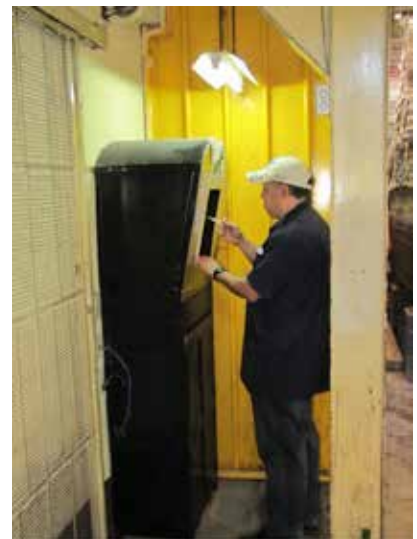
A machine operator updates a job with the barcode scanner through the Shop Floor Data Collection station.
