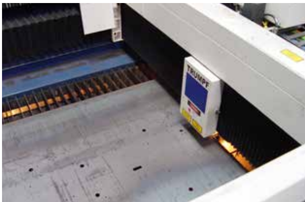
A 4000-watt Trumpf Laser precision cutting carbon steel
