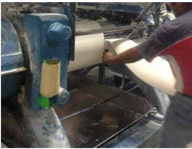
Part of the rubber component mixing process at Archer Advanced Rubber.
