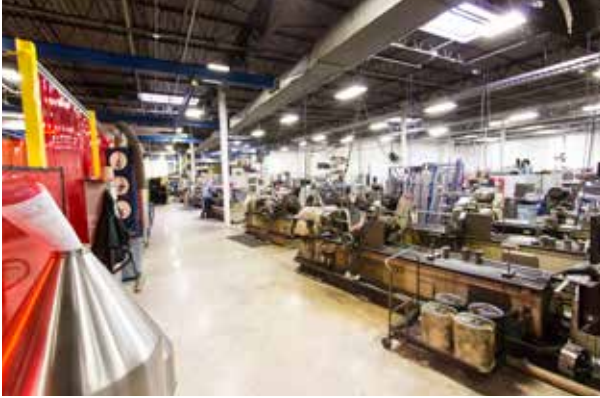
Auger Fab's shop includes a variety of machinery: 6 thread mills, 8 welding booths, 10 manual engine lathes, 12 CNC multiple axis machines, and 3 manual mills
