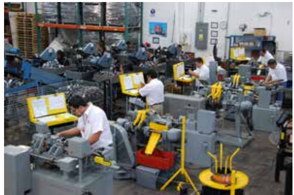
BHI Solutions employees using precision tooling to produce wire forms and fourslides.
