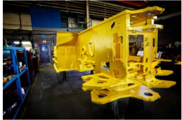
Scooptram frame weldment ready to mount.
