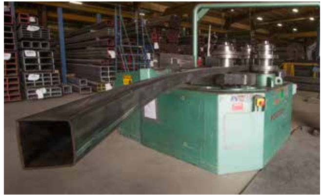
A steel rigging roller at work at the Brunswick Steel facility in Winnipeg, Manitoba.
