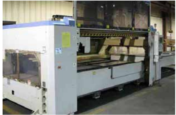
A laser cutter used for cutting large pieces of sheet metal.
