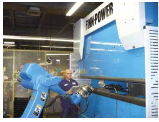
A Concise Industries employee sets up one of the many robotic press brakes.
