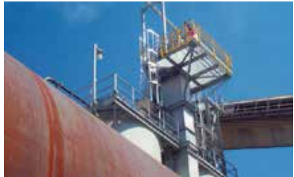
A hot lime bucket elevator.
