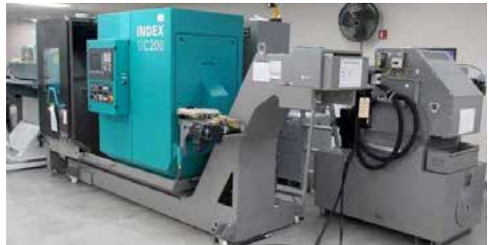
One of Corsair Electrical Connectors’ C200 production turning machines, used to manufacture complex parts.
