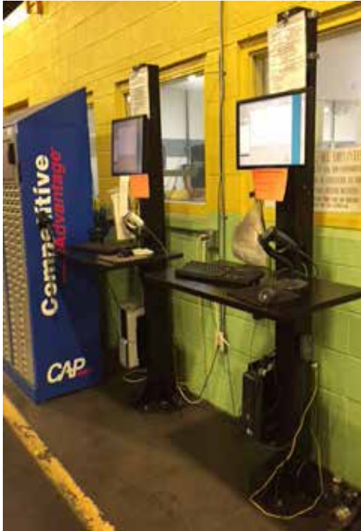
Creed Monarch’s labor collection accuracy and efficiency was significantly improved with the introduction of 14 free-standing Shop Floor Data Collection stations throughout the production floor, in addition to three additional desktop stations in their tool-making and inspection rooms.
