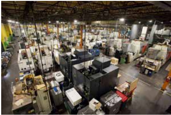
This area at Creed Monarch's facility is comprised of rotary transfer equipment, varied CNC production cells, CNC grinding machines, assembly, final inspection and shipping areas.
