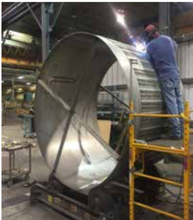
Welder fabricating a large tank.
