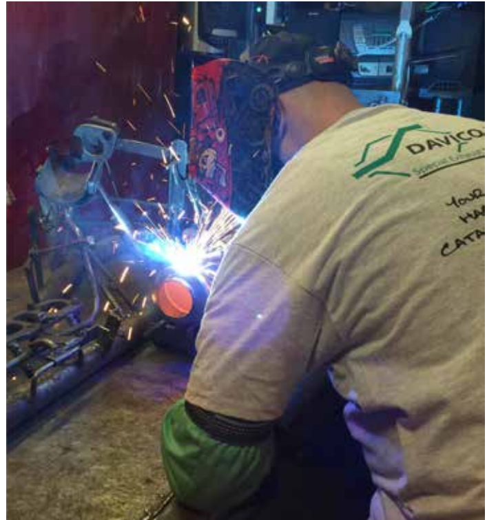
Welding a direct-fit catalytic converter.
