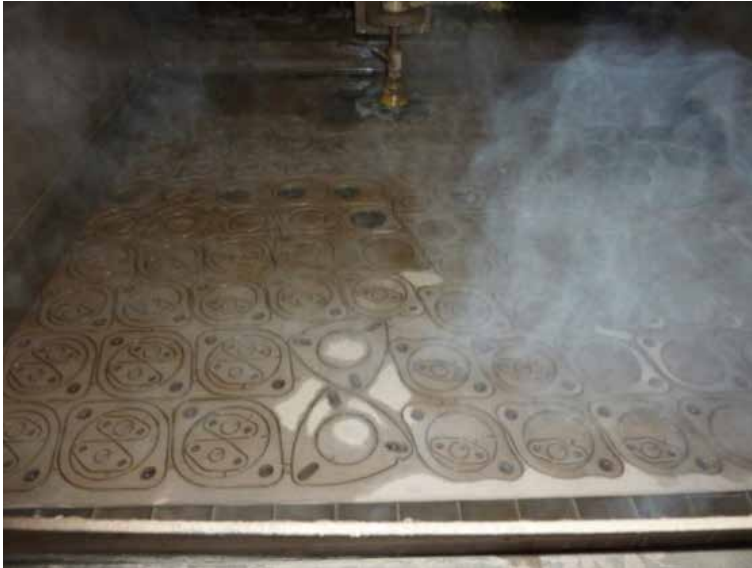
Automotive flanges cutting on a waterjet machine.
