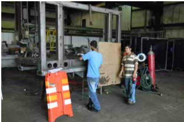
FabCorp production staff work on building a heavily armored military vehicle superstructure.
