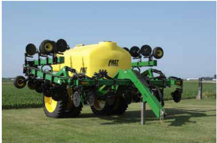
The side-fold applicator is used for narrower transport widths and shorter transport heights
