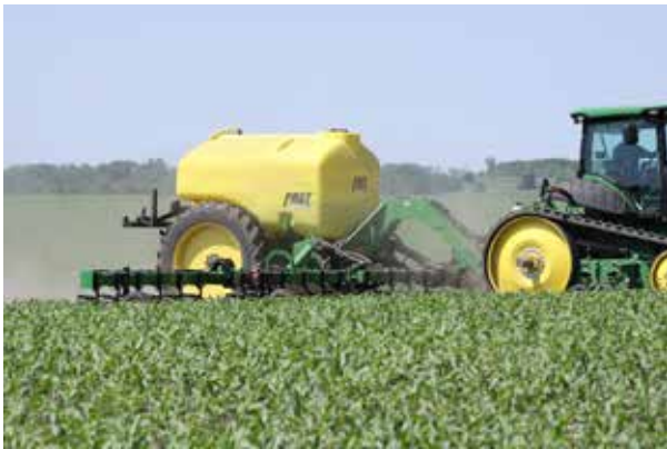
The 8224 Applicator is used to inject liquid fertilizer into the soil.
