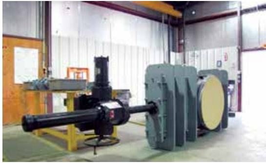
A Fisher Control valve used to control the ethylene oxide flow inside of a process unit.
