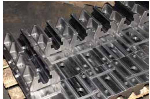
Boring mill jaws produced by H&R Manufacturing & Supply await completion on the shop floor.
