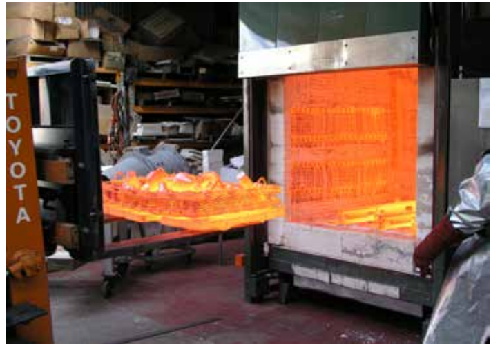
Heat Treatments’ Bogie Hearth Furnace reaches temperatures of over 800 degrees Celsius.
