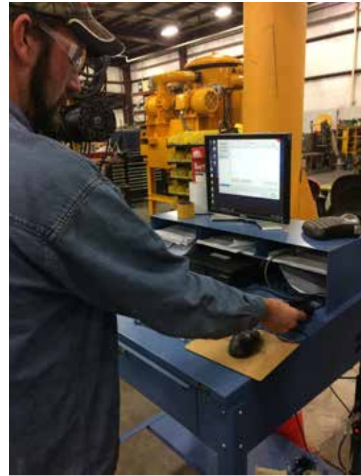
Hi-Vac employee logs himself in on the Shop Floor Data Collection screen using an RFID card in his wallet.
