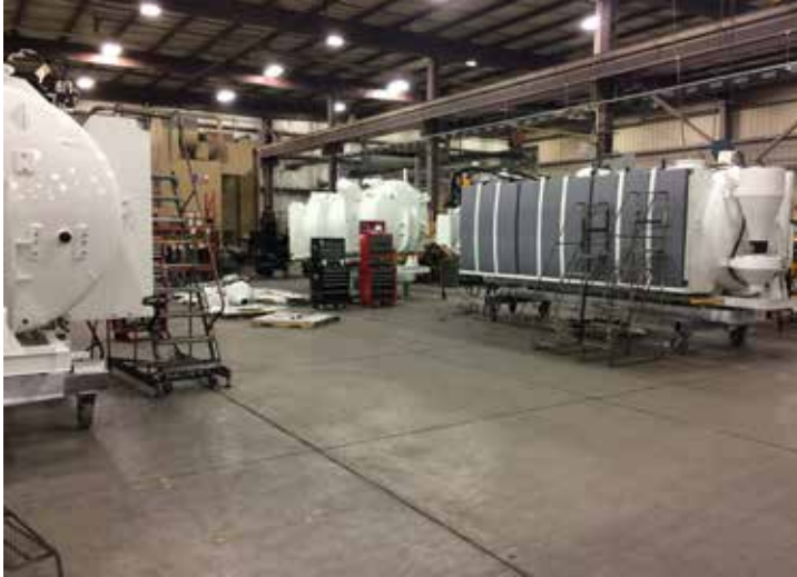
Aquatech debris tanks in various stages of assembly.
