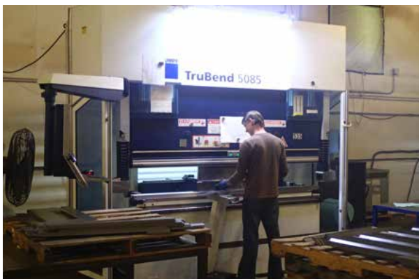
Trumpf TruBend 5085 4-axis at work at ICF Industries.
