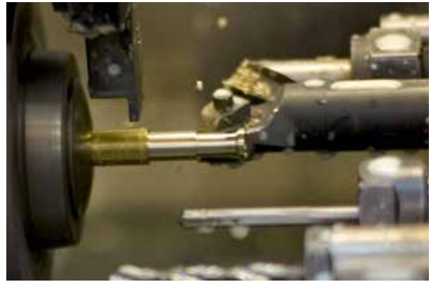
CNC machining part on a CNC machining lathe.
