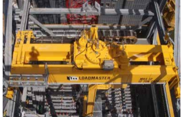
A bridge racker used in the construction of very large assemblies.
