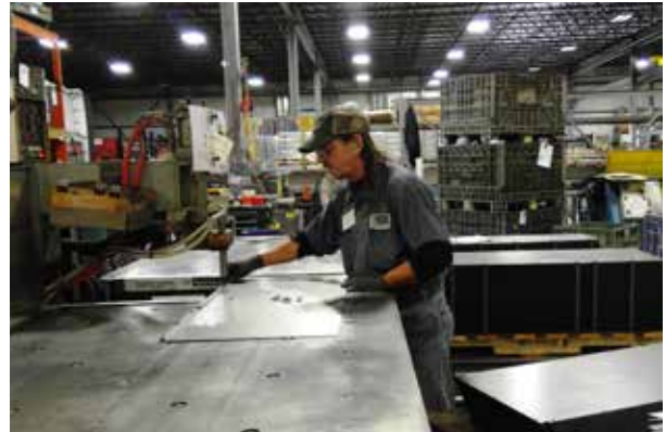
A Louis Industries employee cutting steel.
