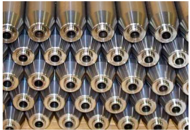
Gun barrels at the beginning stages of production, prior to being hammerforged.
