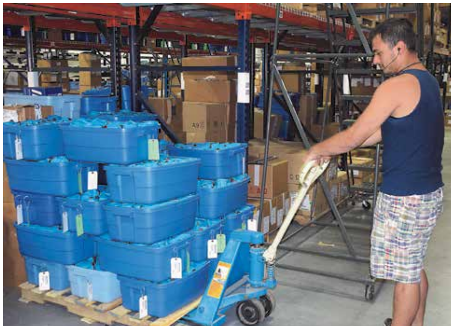
A material handler moves inventory to location. All buckets have inventory barcoded tags with inspection green tags.
