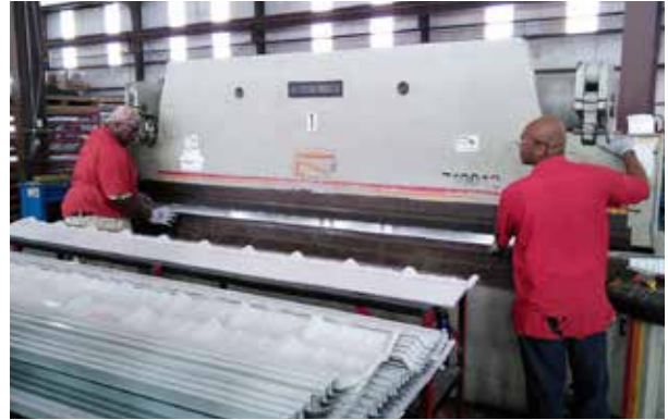
Employees working to break skirts for ridge vents.
