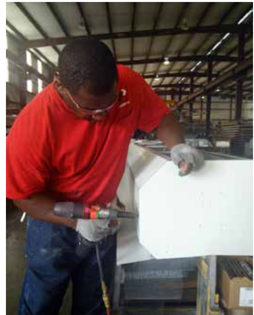
A High Performance Team Leader securing an end cap to a ridge vent.
