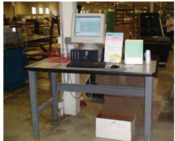
One of the many Shop Floor Data Collection stations located at Milcut's facility.
