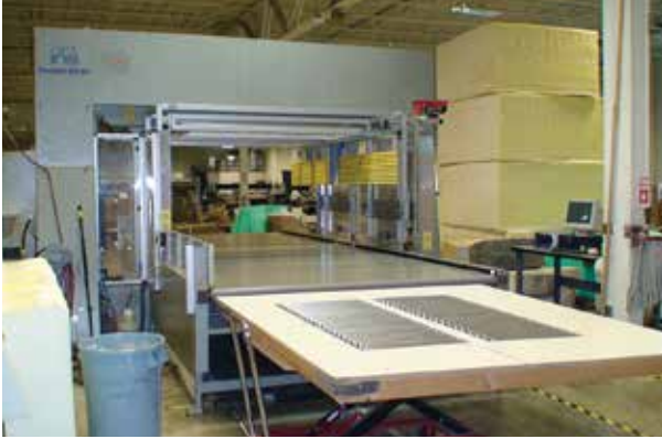
Milcut's two-dimensional profile saw used to cut intricate profiles in flexible or rigid urethane foams and similar materials.
