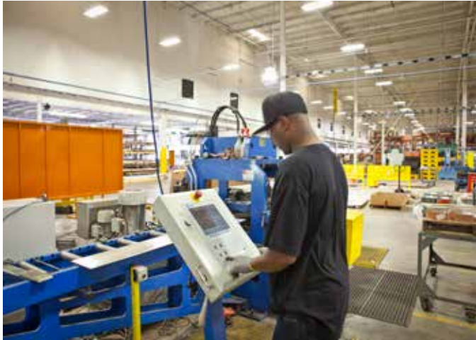
Boschert copper bus bar machine. Punches and cuts of copper in one operation.
