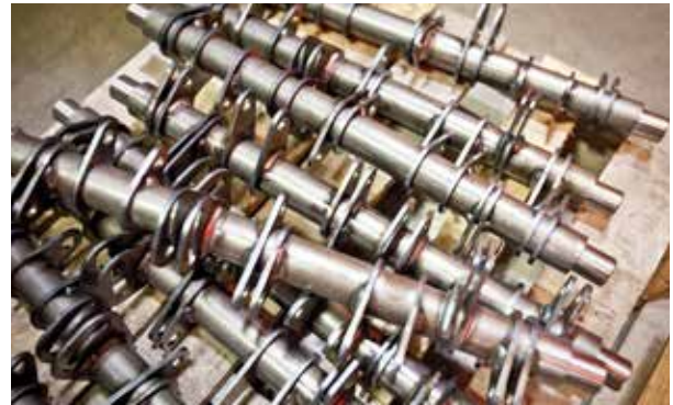
Sample of a welded assembly wheel parts from multiple departments are married together.
