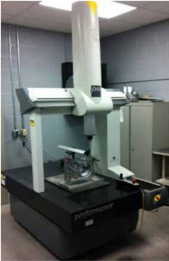
Coordinate Measuring Machine confirming the quality of a part.
