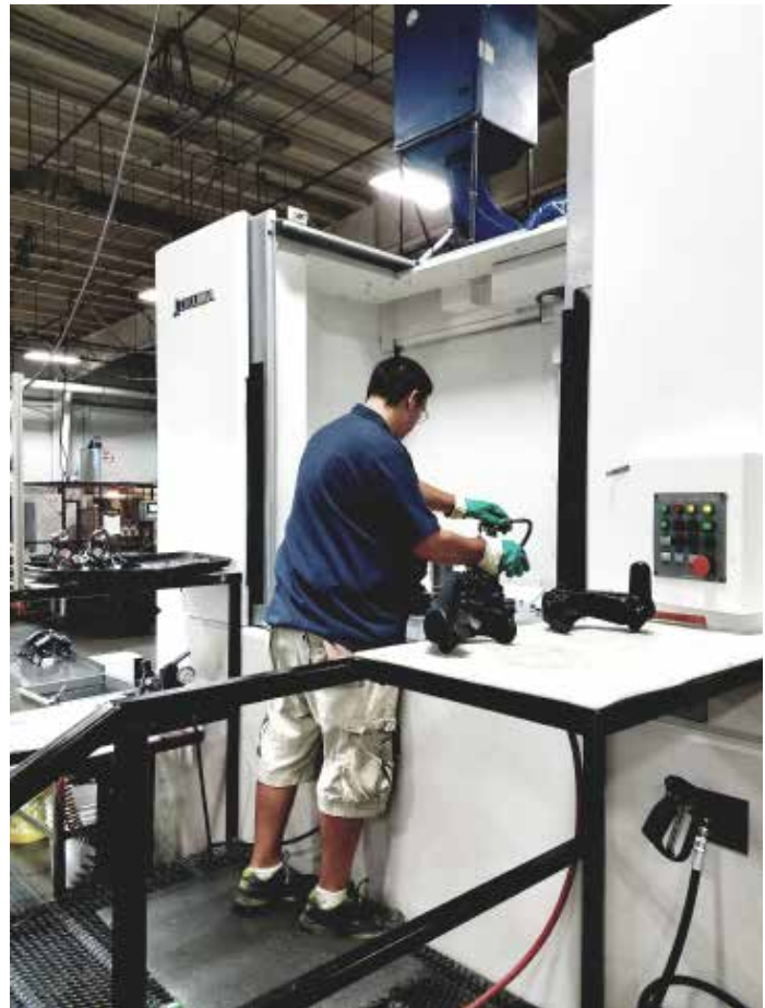
Nowak Machined Products employee loading parts onto an Okuma Horizontal Machining Center.
