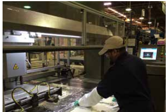
Pacor's moveable head press cutting out parts.
