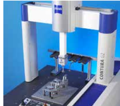
Pazmac uses quality assurance equipment, such as this Zeiss Contura G2 RDS.
