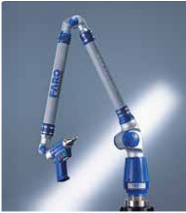
This 2006 Faro CS Platinum Portable Programmable CMM has a laser scanning cad to part comparison 8' arm with 7 axis.
