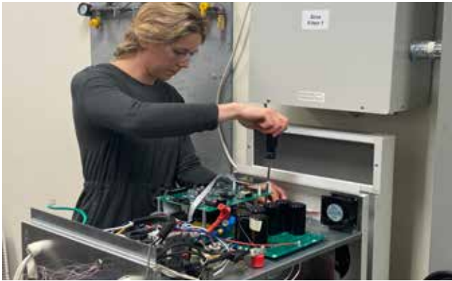
An employee works on the assembly of one of Phase Technologies' Phase Perfect digital phase converters.
