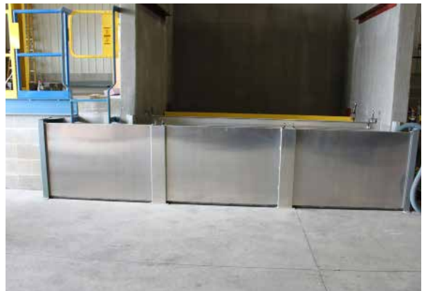
Testing an EzDam flood barrier.
