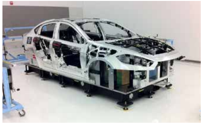
Exceptional welds and fixtures done by Sharp Tooling Solutions on this car body.
