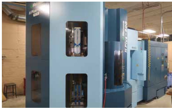
New 15 pallet, 320 tool horizontal machining center, purchased to reduce lead times from 3-4 weeks to 5 days and eliminate 50% of finished goods inventory.
