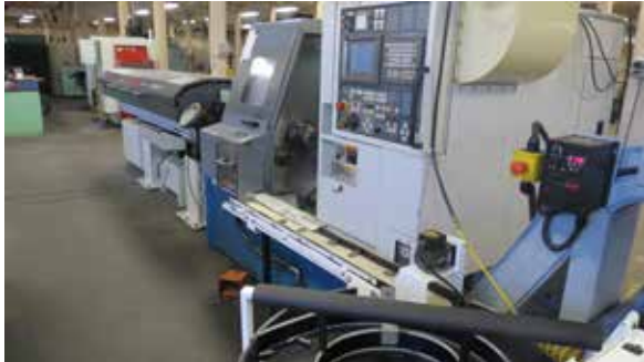
6" lathe with live tooling, barfeeder, and Rotorack parts stocker installed to allow unattended after-hours production.
