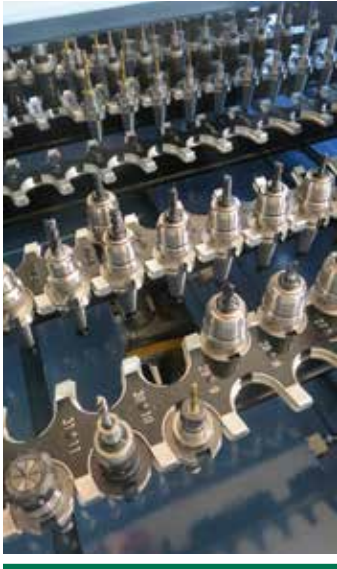
Partial view of the 320 automation tool changer pictured on page 2.
