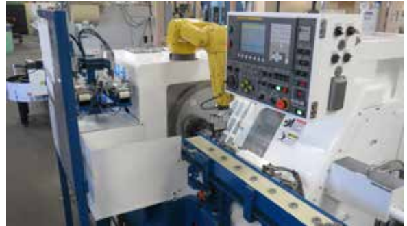
Automated twin spindle lathe purchased to increase capacity and reduce lead time for consumable products. It reduced lead team from 3-4 weeks to 7-10 days and expanded capacity by 200%
