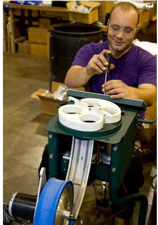
Assembly of a Coach tennis ball machine.
