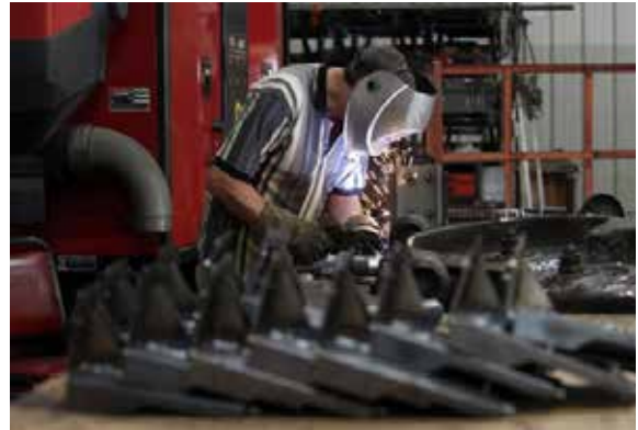
Staber's employee welding the base frames for their washing machines.
