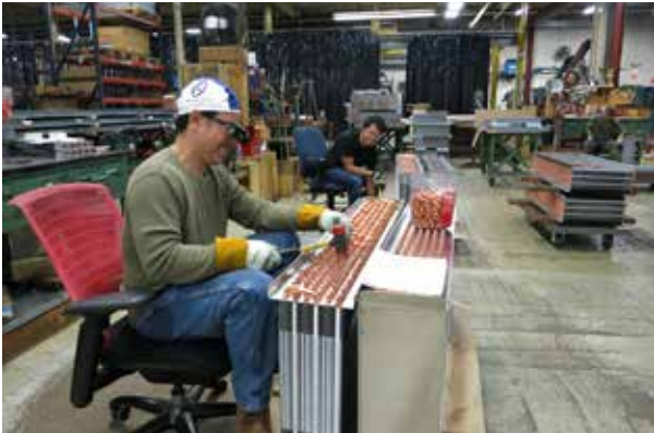
Super Radiator Coils employee hammering together two pieces of coil to make one solid part.
