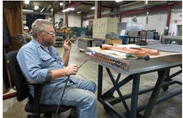
Another Super Radiator Coils employee welding coils together before completing a project.
