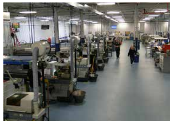
The main shop floor, which contains 27 Star CNC Swiss screw machines.
