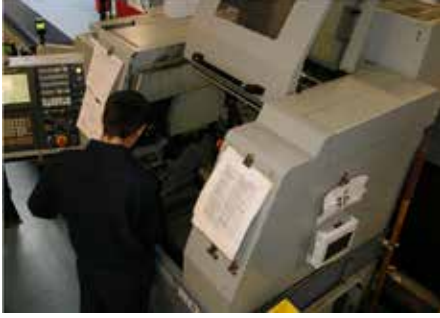
Setting up a 20-mm diameter capacity Star SR-20R-II, which is used for complex parts.
