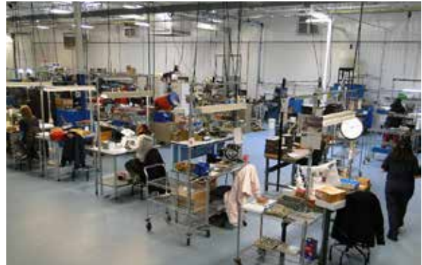
The secondary/finishing department, where parts are washed, counted, deburred, and undergo secondary operations.
