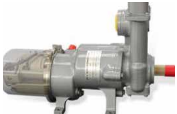
A finished Thomas Instrument Gear Box Assembly.
