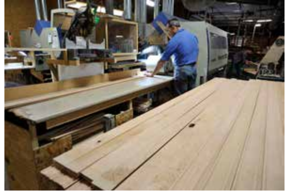
Two high precision, HSK spindle, Weinig moulders to produce moldings.
