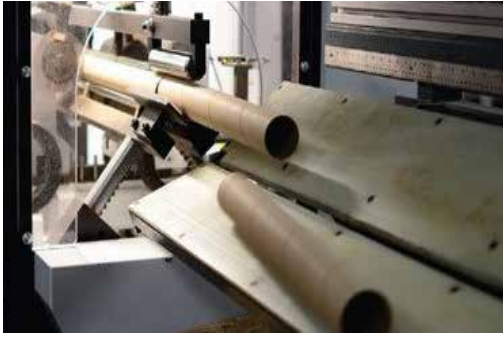
One of Western Container's Zenith 300/2 in-line cutters.
