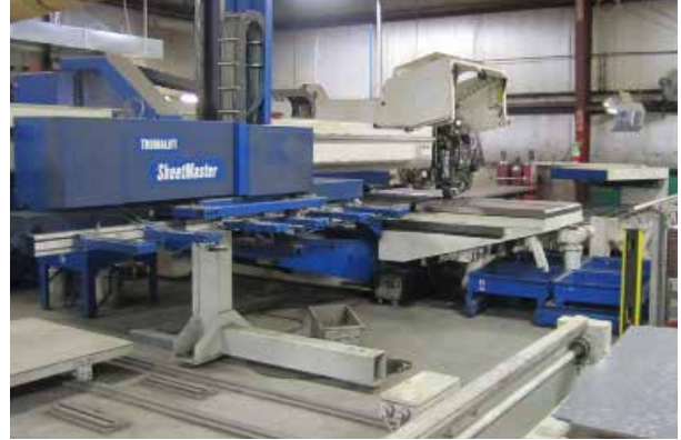
A Trumpf laser punch combo that cuts different shapes with the laser and drops them into separate material pans.
