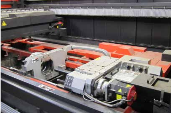
Zephyr's new 4000-watt laser with rotary can do any flat sheet up to 1", while the rotary can laser any structural steel or tube up to 8".
